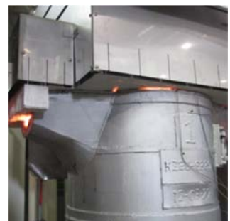
Figure 3: Kanthal ladle heater system
