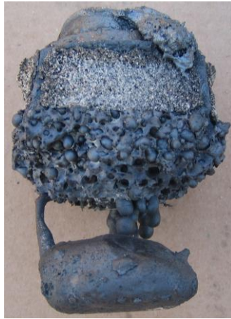
Figure 8: Filter is clogged by leaking metal from the nozzle
