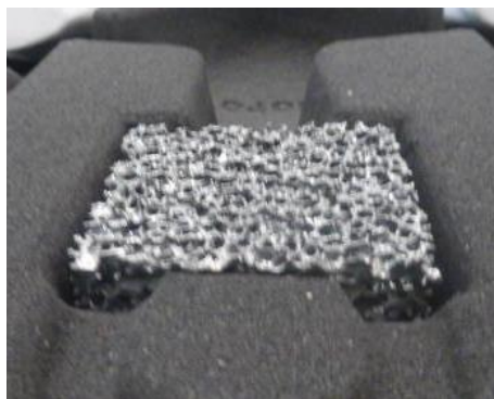
Figure 7: Drowned filter under the parting line – By pass present
