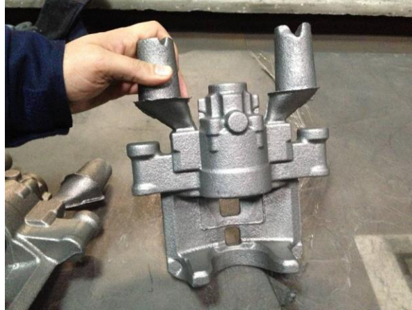
Figure 3: Sound casting with KALMINEX ZP 4/7K exothermic feeder
